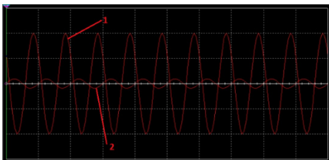
Figure 9. The oscilloscope display for the low-pass filter
