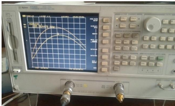
Figure 9. Display of the results of impedance measurement using VNA.
