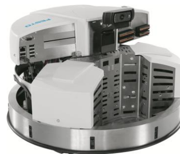
Figure 1. Mobile robot system Robotino ®
